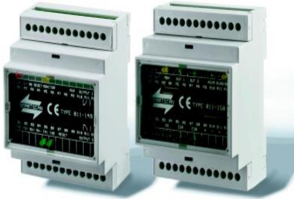
Smartscan Multifunction Safety Unit (MFU) provides relay output switching options. They are typically used with the Smartscan 1000 Series Light Curtains where a relay output option is required as opposed to the two fail-safe electronic output switches provided by the light curtain.
